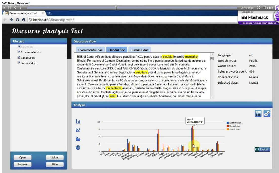
Figure 1: The DAT interface: in the left window appear the selected files, in the middle window – the text from the selected file, and in the right window, information about the text (language, word count, dominant class, etc.). Below, a plot chosen from a range of graphical styles is displayed. By selecting a specific class in the middle window, all words assigned to that class are highlighted in the text.
